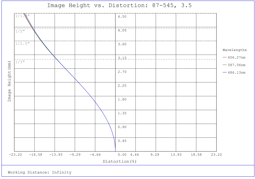
#87-545, 3.5mm, f/2 Ci Series Fixed Focal Length Lens, Distortion Plot
