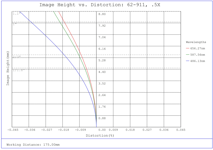
#62-911, 0.5X CobaltTL Telecentric Lens, Distortion Plot
