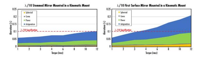
A comparison of the aberrations introduced to a  $\lambda/10$  Stemmed Mirror and a  $\lambda/10$  First Surface Mirror when mounted in a kinematic mount. As shown, a Stemmed Mirror stays within  $\lambda/10$  specification up to 12 inoz of torque ("hand-tight") while a First Surface Mirror becomes out of specification with a surface flatness of  $\lambda/5$ .
