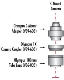
Recommended 50-75mm spacing for optical filters, beamsplitters, or in-line illumination
