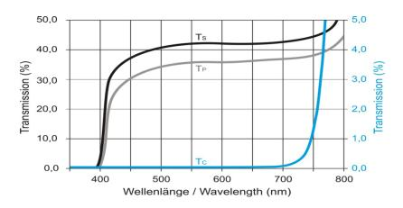
The XP42HE is a sheet polarizer with high transmission of light and polarization of 400-700nm. This polarizer has the highest contrast as it allows the least amount of visible light to pass. The polarizer is typically used for high-end applications within the short-wave spectral field.
